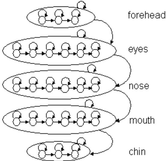
Fig. 2. Embedded HMM state structure for face recognition.
